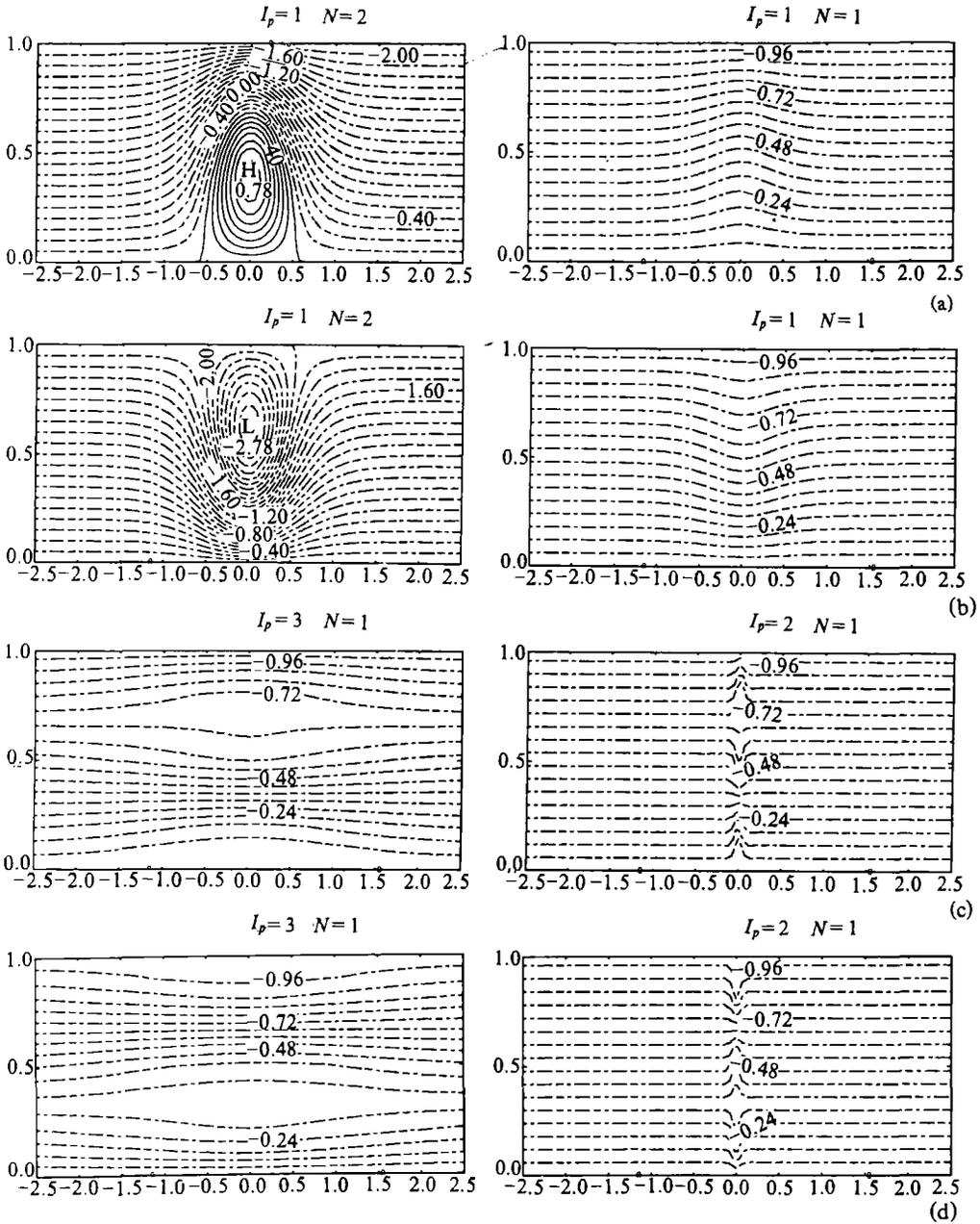
Fig. 1. The streamline patterns of solitary Rossby wave for meridional wavenumber  $m=1$  and 3. ( $F_r=0.5$ , D-shear pattern). (a) Anticyclonic horizontal shear and southern slope of topography; (b) Cyclonic shear and southern slope; (c) Anticyclonic shear and northern slope; (d) Cyclonic shear and northern slope. (a) and (b) :  $m=1$ , barotropic modes; (c) and (d) :  $m=3$ , upper figures — baroclinic modes 1, lower figures — baroclinic modes 2.
