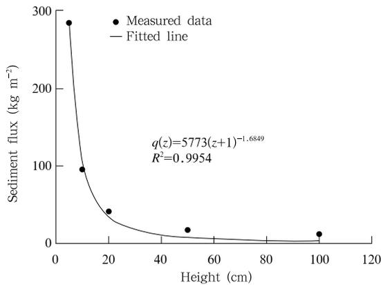
**Fig. 5.** Sediment flux at different heights above the soil surface.
