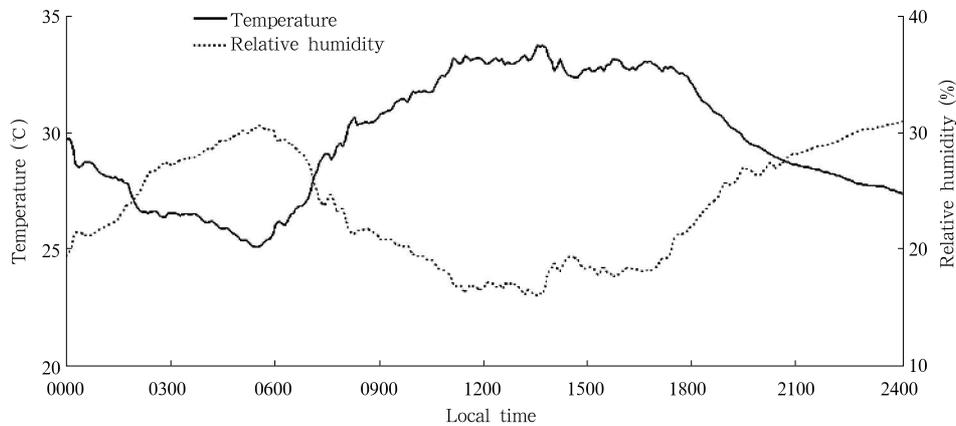
Fig. 3. Temperature and relative humidity measured at 1.5-m height.
