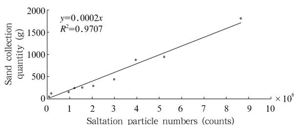
**Fig. 1.** Saltation particle numbers and sand collection quantity trapped by the BSNE.
