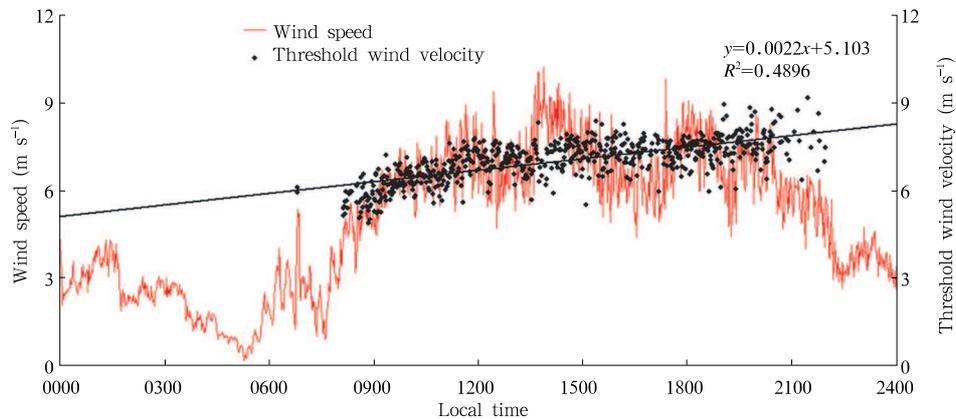
Fig. 4. Wind speed at 2-m height and threshold wind velocity.
