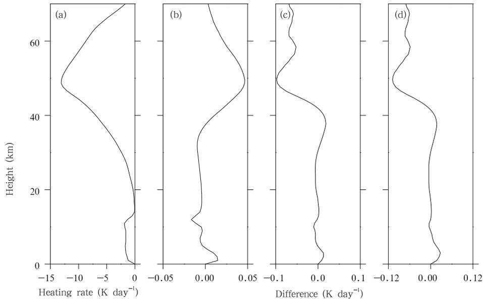
**Fig. 2.** Heating rate calculated by HITRAN08 and the differences of heating rates between other HITRAN versions and HITRAN08 for MLS atmosphere. (a) The heating rate calculated by HITRAN08; the relative difference between (b) HITRAN04 and HITRAN08, (c) HITRAN2K and HITRAN08, and (d) HITRAN96 and HITRAN08.
