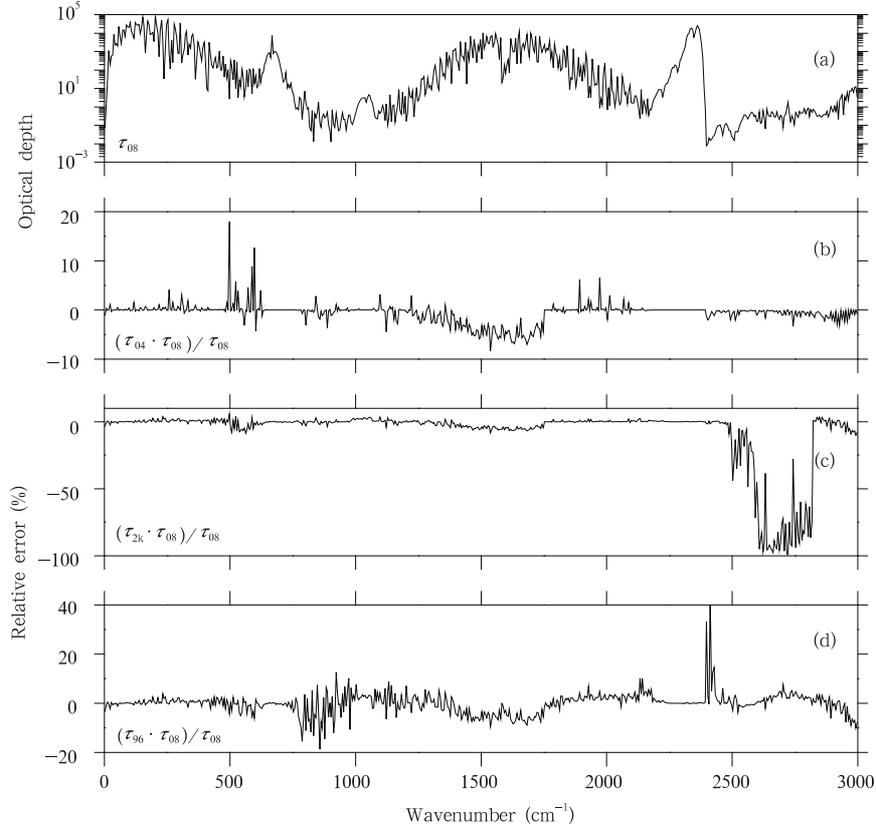
**Fig. 1.** Comparison of optical depth in the long-wave regime from 0 to 3000  $\text{cm}^{-1}$  for MLS atmosphere. All the curves have been smoothed to have a  $5\text{-cm}^{-1}$  resolution. (a) The optical depth calculated by HITRAN08; the relative difference between (b) HITRAN04 and HITRAN08, (c) HITRAN2K and HITRAN08, and (d) HITRAN96 and HITRAN08.
