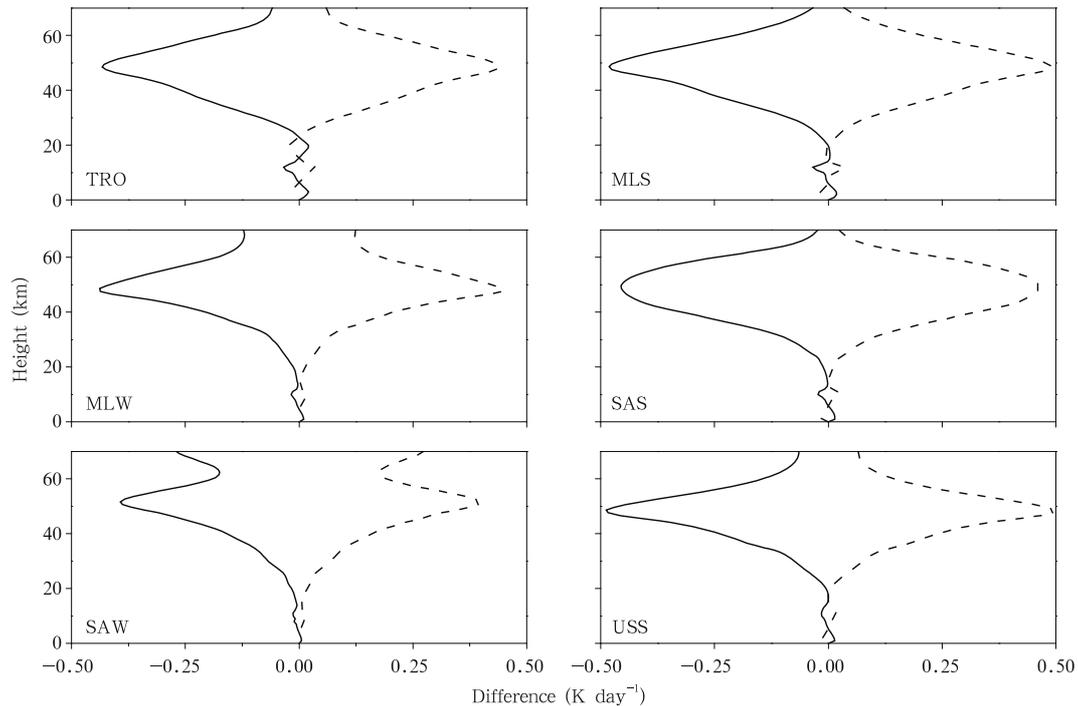
**Fig. 4.** As in Fig. 3, but for heating rate. Solid lines represent the bias caused by the minimum value of the uncertainty of intensity and air-broadened half-width, and dashed lines denote the bias caused by the maximum value of them.
