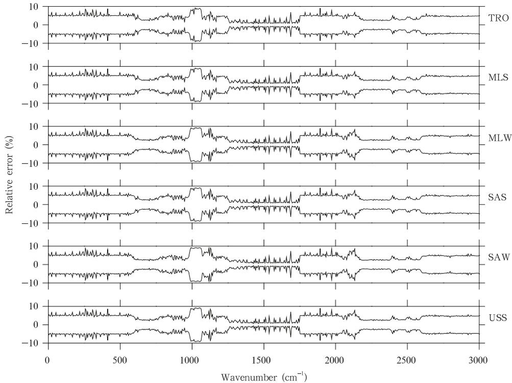
**Fig. 3.** Uncertainties of optical depth for six typical atmospheres. Top to bottom panels are for tropical (TRO), midlatitude summer (MLS), midlatitude winter (MLW), sub-arctic summer (SAS), sub-arctic winter (SAW), and United States Standard (USS) atmospheric profiles, respectively.
