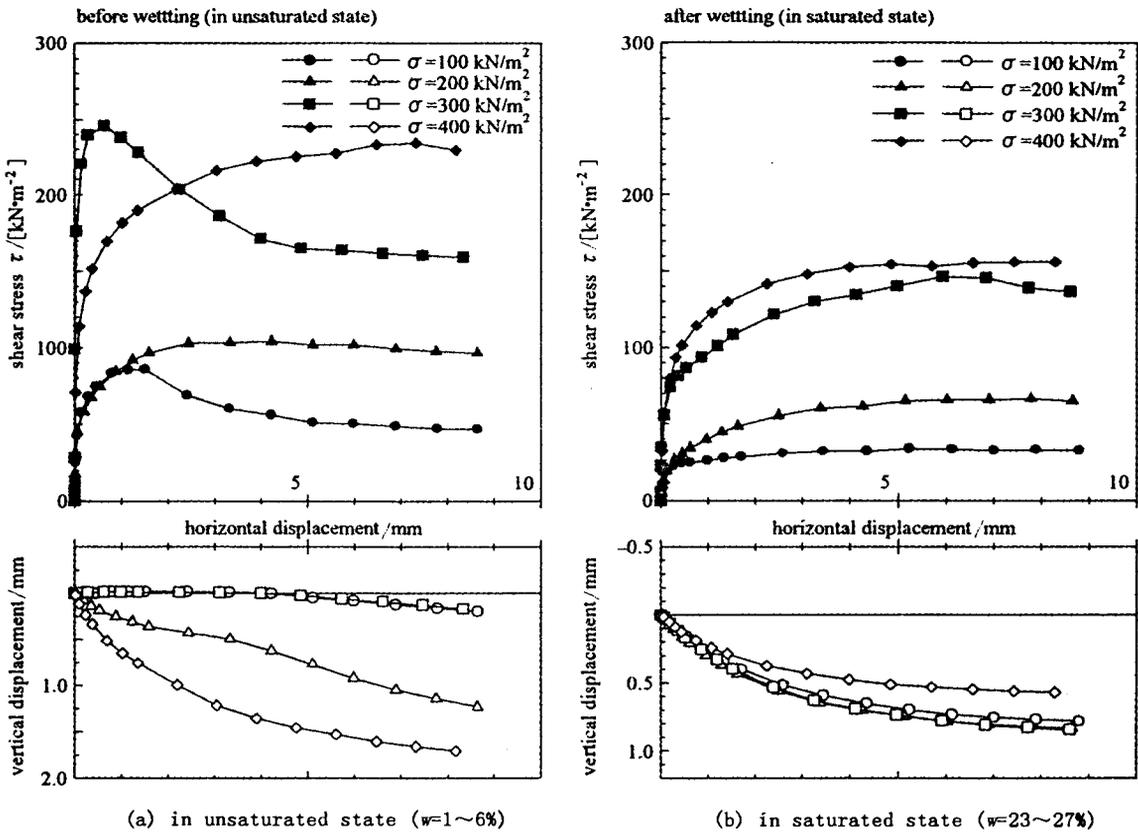
Fig. 3 Shear stress-verticle displacement-horizontal displacement curve for the undisturbed specimen of the non-irrigated soil .
