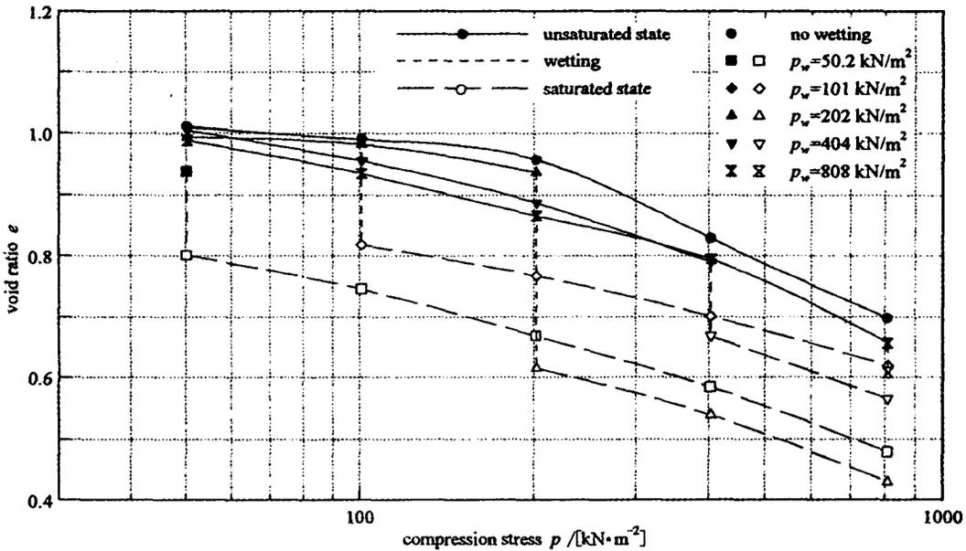
Fig. 2  $e$ - $\log p$  curves for the one-dimensional response-to-wetting test using the remolded specimen of the non-irrigated soil.
