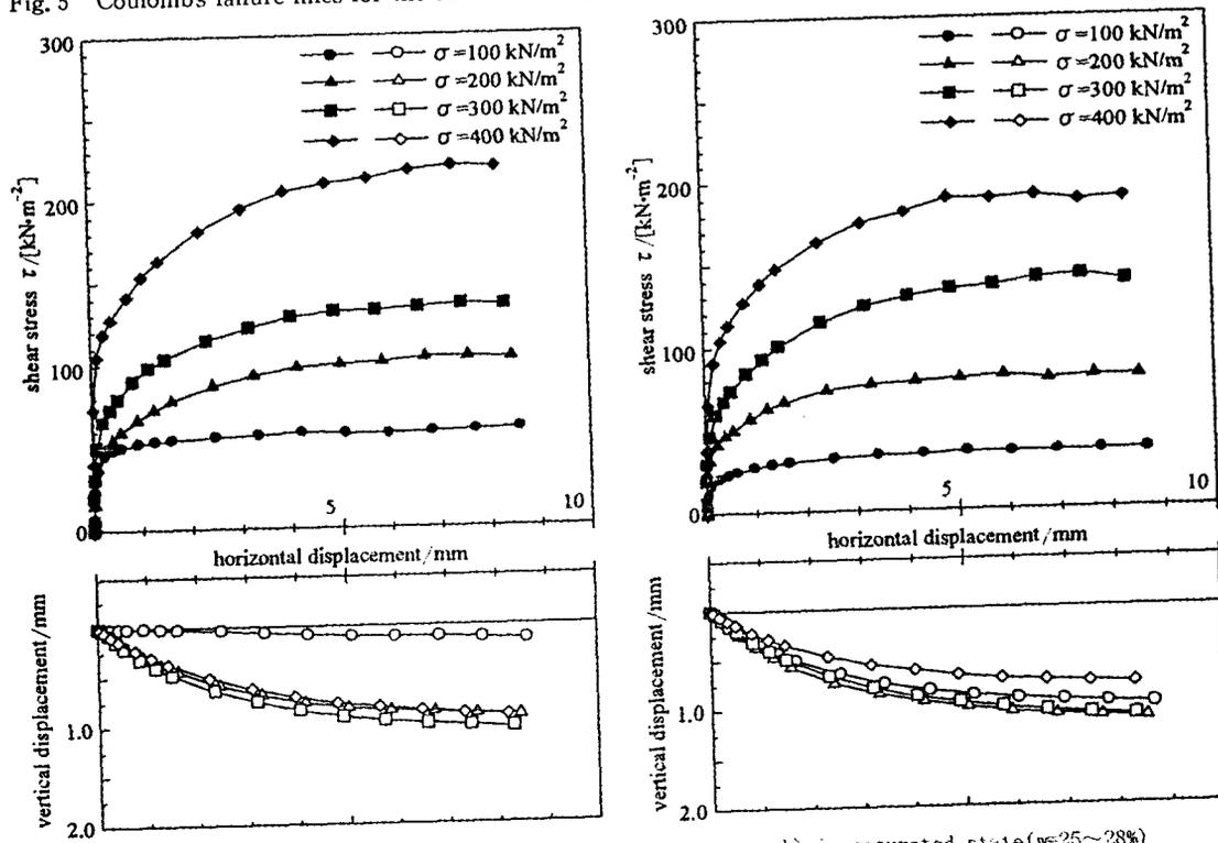
(a) in unsaturated state (w=5%) (b) in saturated state (w=25~28%)
