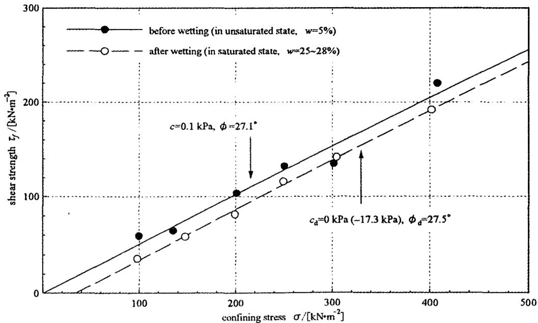
Fig. 7 Coulomb's failure lines for the remolded specimen of the non-irrigated soil .
