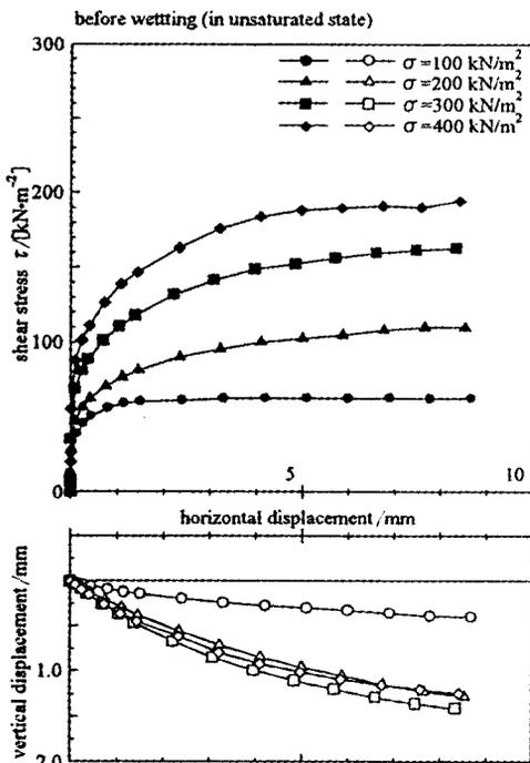
Fig. 4 Shear stress-verticle displacement-horizontal displacement curve for the undisturbed specimen of the irrigated soil in unsaturated state( $w=15\sim16\%$ ).
