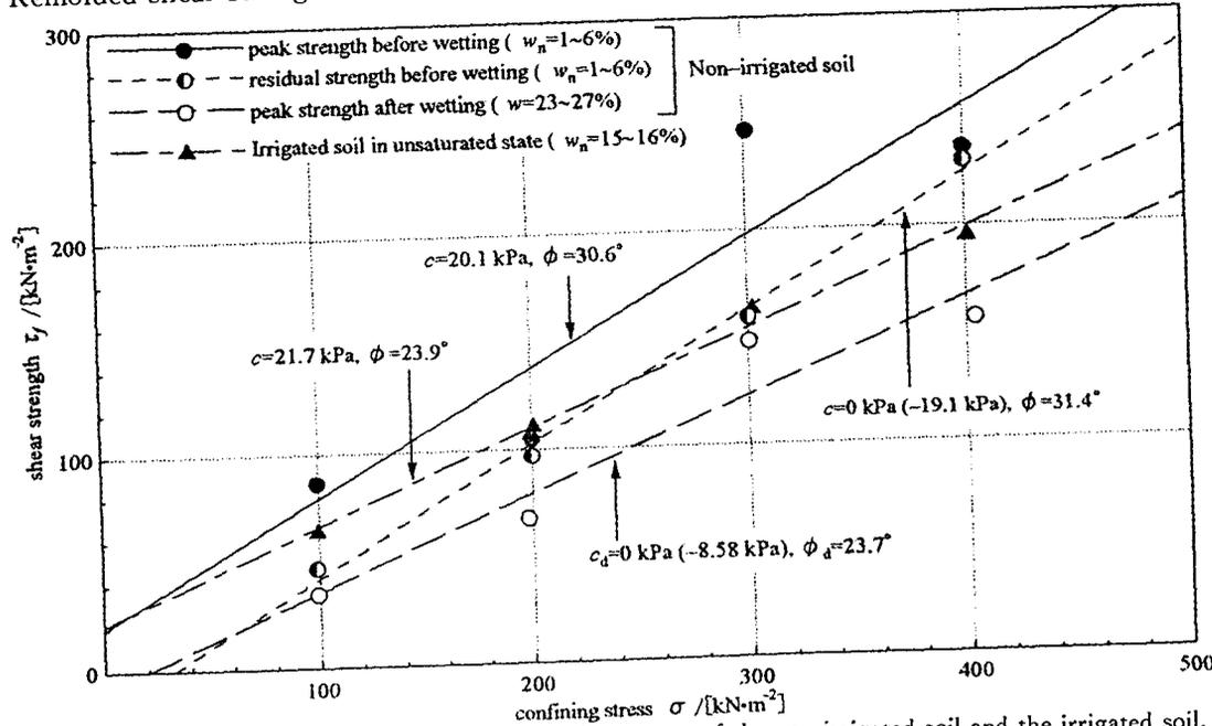
Fig. 5 Coulomb's failure lines for the undisturbed specimen of the non-irrigated soil and the irrigated soil.
