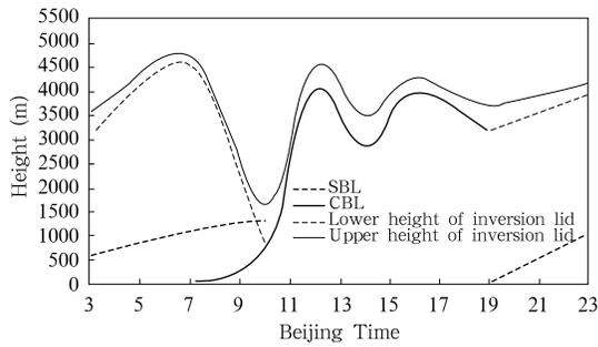
**Fig.2.** Diurnal variation characters of the depth of atmospheric thermodynamic boundary layer in a typical sunny day (May 29, 2000) in Dunhuang region.
