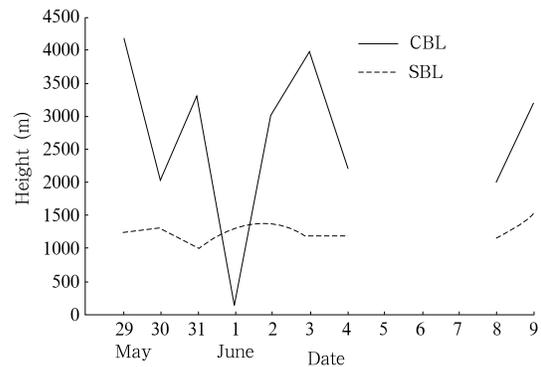
**Fig.3.** Daily variation of maximum depth of convective boundary layer and stable boundary layer from May 29 to June 6 in Dunhuang region.
