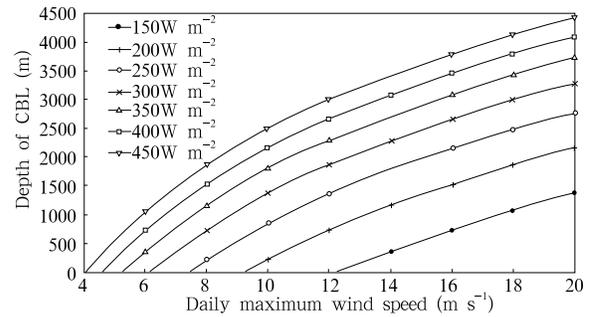
**Fig.12.** Dynamic change of the daily maximum depth of CBL calculated from Eq.(6) with daily climax sensible heat flux and daily maximum wind velocity.
