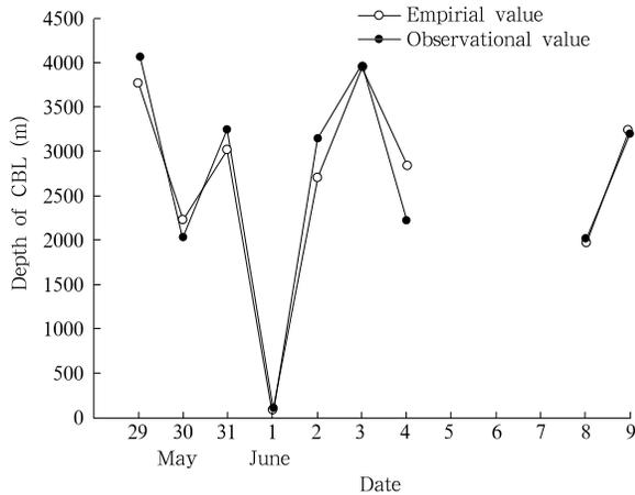
**Fig.10.** Comparison of observed data with the daily maximum depth of CBL calculated from Eq.(6) during May 29 to June 9.
