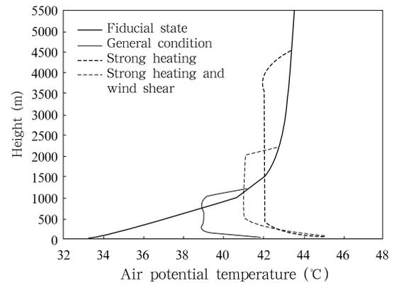
**Fig.8.** Illustration of strong surface buoyancy flux and strong wind shear's influences on development of CBL.
