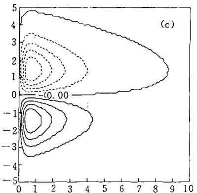
Fig. 7. The structure of the physical fields after meridional semi-geostrophic adaptation. The vertical axis is meridional length, the horizontal axis is zonal length. (a) The pressure field. (b) The zonal velocity field. (c) The meridional velocity field. In the computation,  $\alpha_1 = \alpha_2 = 0.02$ .
