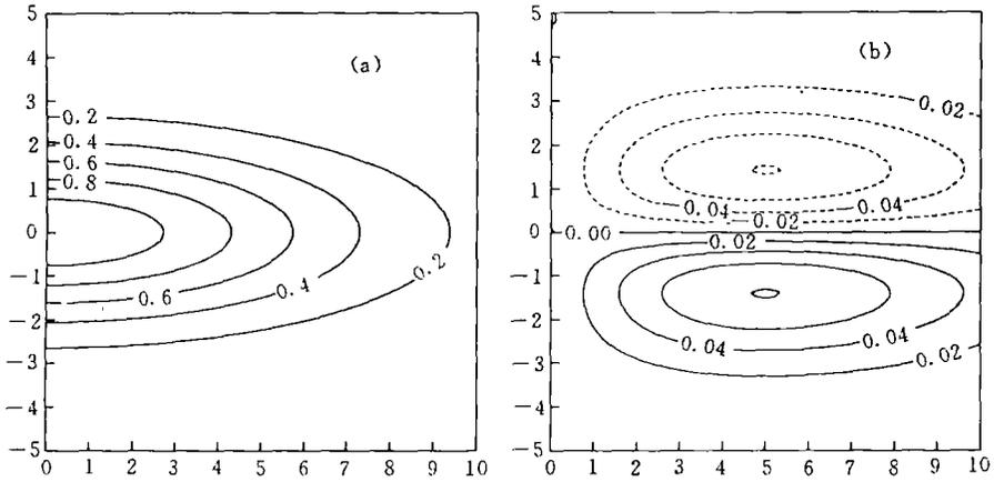
Fig. 4. The structure of the physical fields after zonal semi-geostrophic adaptation. The vertical axis is meridional length, the horizontal axis is zonal length. (a) The pressure field. (b) The meridional velocity field. In the computation,  $\alpha_1 = \alpha_2 = 0.02$ .
