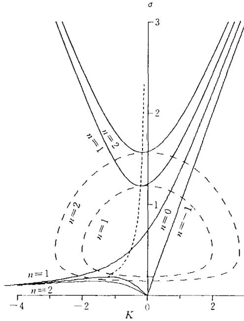
Fig. 1. Dispersion curves for equatorial waves. The vertical axis is the frequency and the horizontal axis is the east-west wavenumber. The curve labeled 0 corresponds to the mixed Rossby-gravity wave. The upper curves labeled 1 and 2 are the first two gravity wave modes and the corresponding lower curves are the first two Rossby wave modes. The straight line labeled -1 corresponds to the Kelvin wave. The dashed curves are the boundary waves.
