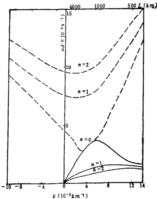
Fig. 1. Dispersion relation of the tropical oceanic wave when  $\tilde{S}_y=3.3 \times 10^{-6} m^{-1}$ . The dashed lines represent the inertia-gravitational wave, while the solid lines represent slow wave.
