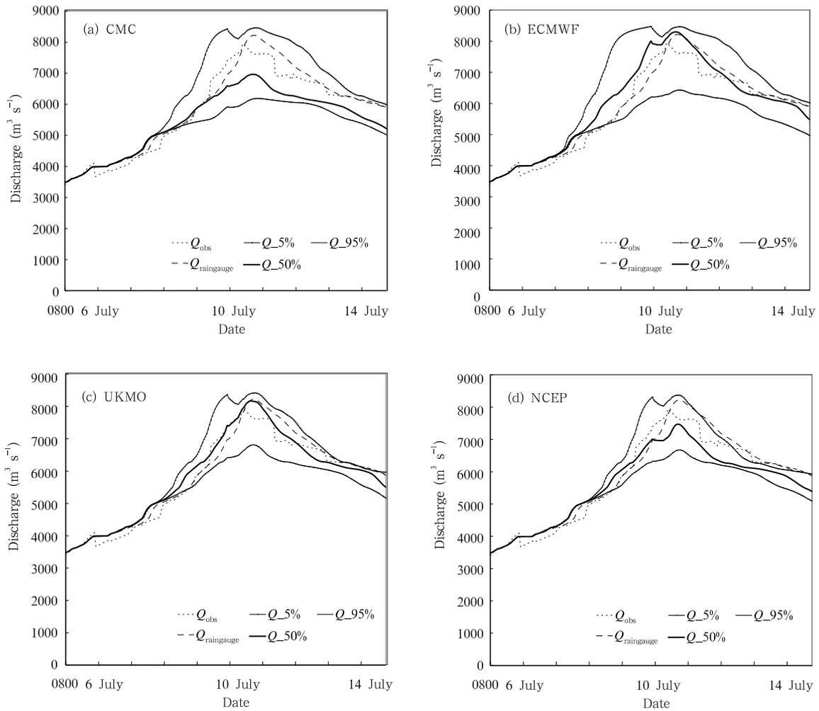
Fig. 4. Ensemble forecast discharges issued on 6 July 2007 from the coupled atmospheric-hydrologic-hydraulic model driven by the TIGGE data of the four centers (CMC, ECMWF, UKMO, and NCEP) in comparison with observation.
