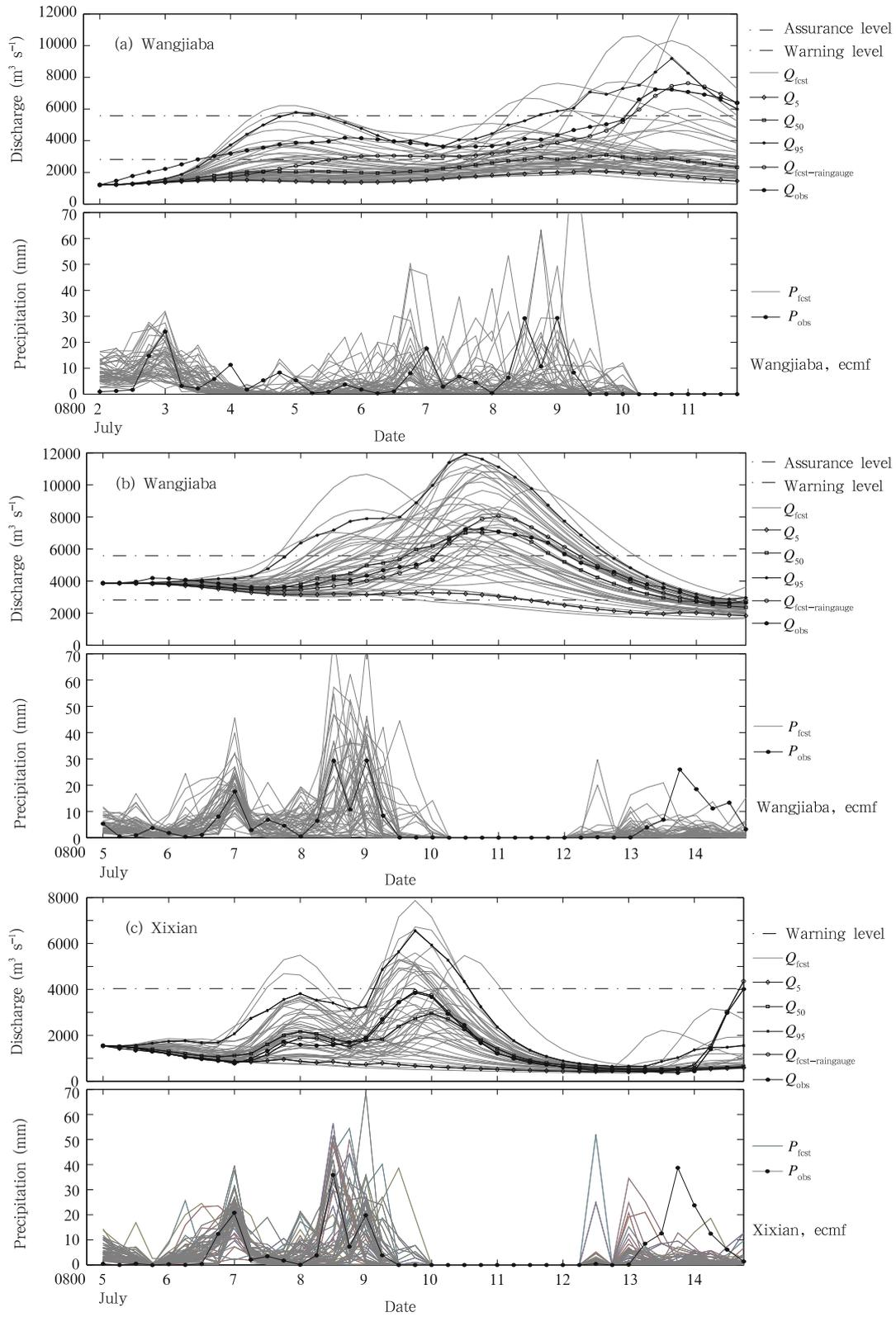
**Fig. 1.** Ensemble precipitation forecasts issued on (a) 2 and (b, c) 7 July 2007 by ECMWF (lower panels) and ensemble forecast discharges (upper panels) in comparison with observation. (a) and (b) Wangjiaba station, and (c) Xixian station.
